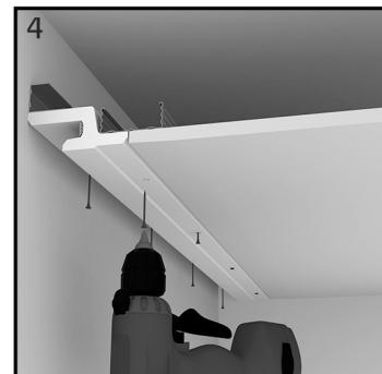
fasten the profile with plasterboard screws at the suggested points
