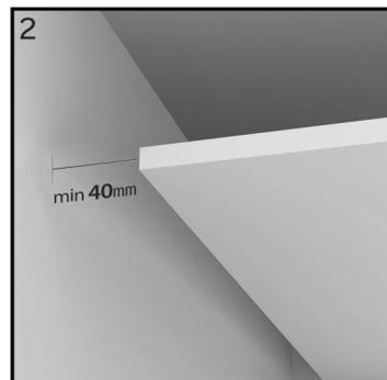
define the desired distance between the plasterboard and the wall
