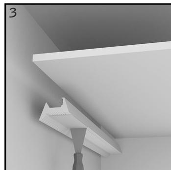
apply joint filler on the bottom of the profile
