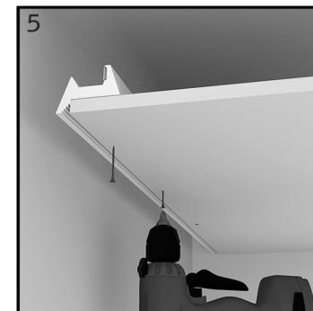
fasten the profile with plasterboard screws (optional)
